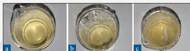
Figure 2. Aloe gel obtained from the edible juice. (a) 2%, (b) 3% and (c) 4% of carboxymethylcellulose.
